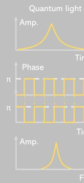
Considering a coherent pulse  $f(t)$ , after a periodic time phase modulation, the frequency spectrum  $F(\omega)$  will be separated to orders of sidebands  $F'(\omega)$ , which can be seen as:
