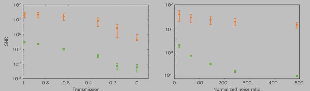
Fig. 6 | SNR comparison for varying transmission rate
