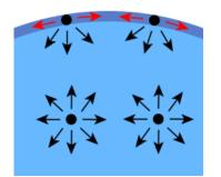
If the interface is curved (such as the surface of a water droplet), or if the surface tension varies with direction, then a single scalar  $\gamma$  is not sufficient to describe all the forces. In such cases, we introduce the **surface stress tensor:**
