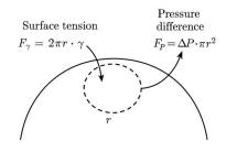
If the small patch is part of a spherical surface, then the local radius of curvature is the sphere's radius R:
